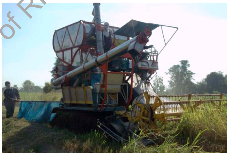
Fig. 1 Thai designed rice combine harvester
